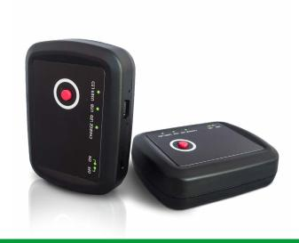
The Tag is an active mobile locator. Its position and ID is reported within configurable refresh rate. The Tracked objects need to be equipped with this device.
