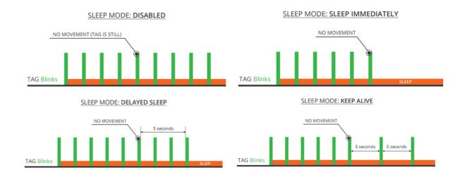
Disabled - Tag send blink message regularly and movement detection is inactive.
